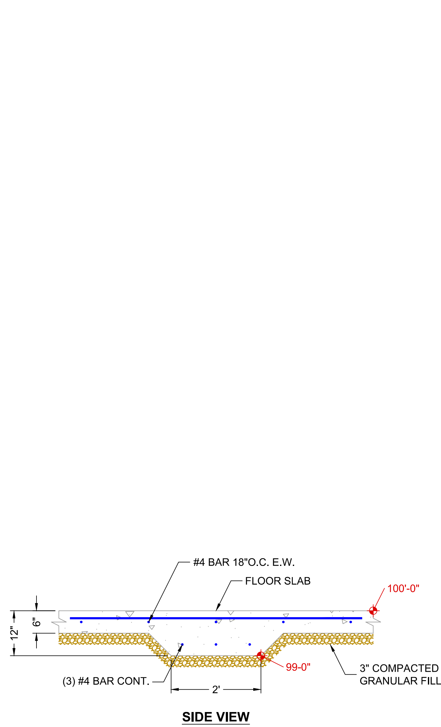
I THICKENED FOOTING AT FRAMED WALL NOT TO SCALE
